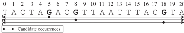
Fig. 3. Algorithm MFILTER: checking candidate occurrences of the RE Q = (G|T)A^*GA^*T^* using necessary factor G , shown in bold font.
